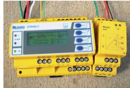
importance that the photovoltaic system is permanently monitored in order to display the occurrence of residual currents as early as possible so that the problem can be solved as soon as possible.
