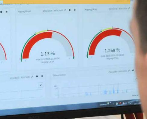
Powerscout® is a web and widget-based software for data management, analytics and effective visualisation. Powerscout® integrates data from Bender RCM, PEM, IPS, UPS, IMDs and third-party devices to help detect malfunctions at an early stage.
