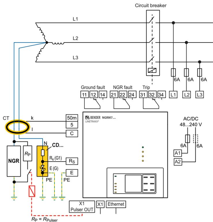
**i** The "N" connection of the CD-series coupling device should be as close to the transformer star point as possible. An intermediate relay may be required between the power contactor of the pulser and the digital output at X1 of the FP200-NGRM.
