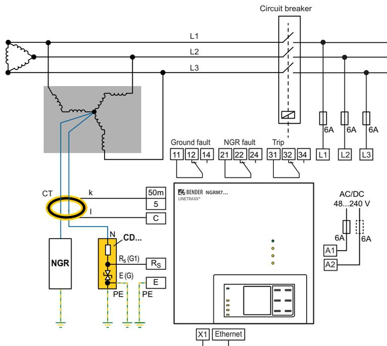
**Measuring current transformer connection**
