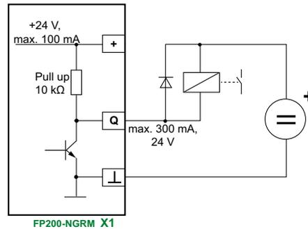
Connection to Q1, Q2: external relay or PLC.
