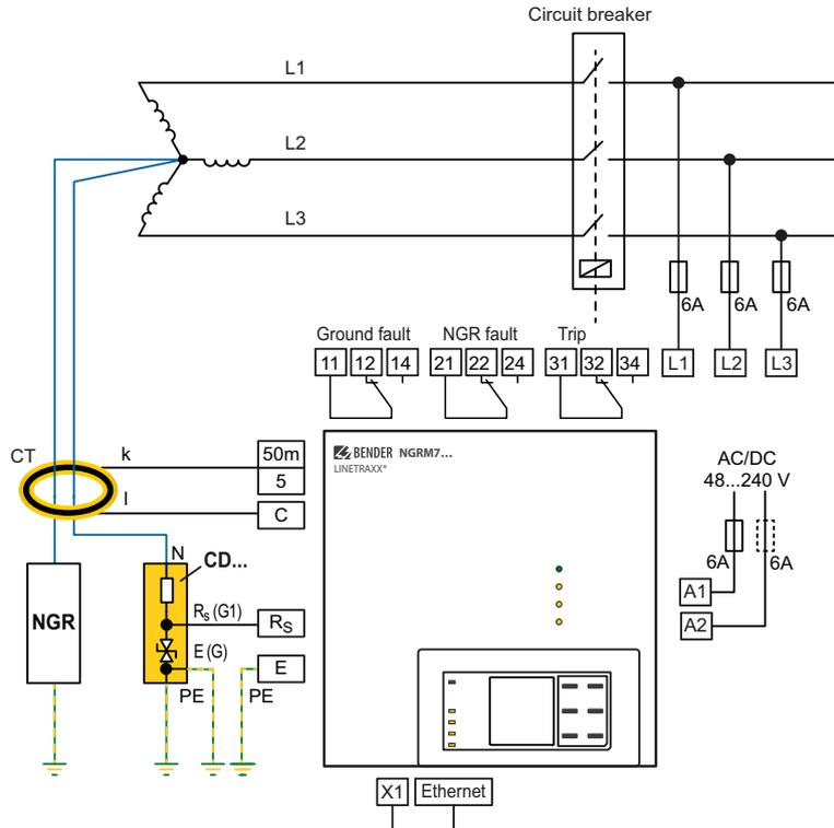
**i** The "N" connection of the CD-series coupling device should be as close to the transformer star point as possible.
