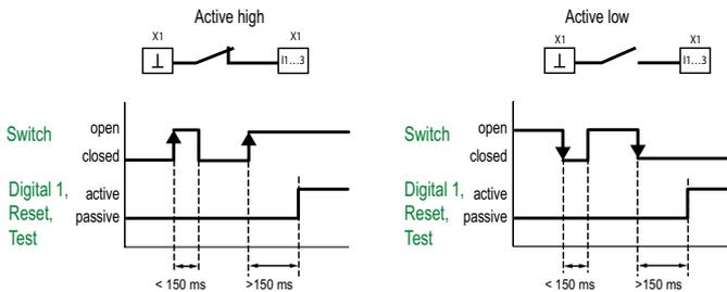
Input I1...3: Potential-free contact to common or 0 V and 24 V in conjunction with a PLC
