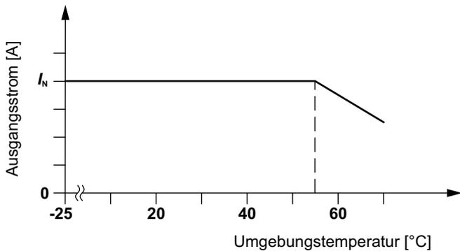
At an ambient temperature of up to +55 °C the device supplies the continuous output current  $I_N$ . In the case of ambient temperatures above +55 °C the output power must be reduced by 2.5 % per kelvin increase in temperature. The device does not switch off at ambient temperatures above +70 °C or thermal overload. The output power is reduced as much as necessary to provide device protection. After it has cooled down, the output power is increased again.
