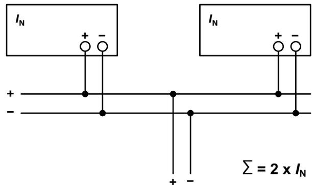
For  $n$  devices connected in parallel, the output current can be increased to  $n \times I_N$ . Parallel connection for increasing power is used when extending existing installations. A parallel connection is recommended if the power supply does not cover the current consumption of the most powerful load. Otherwise, the loads should be divided between individual devices that are independent from one another.
