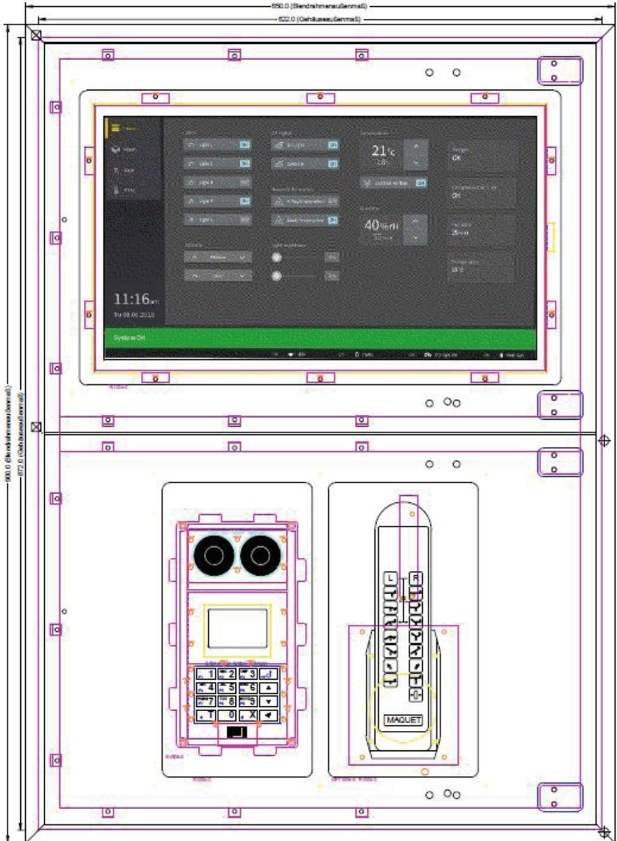
Fig. 2-3 CP921-F with two front plates in bezel frame enclosure.
