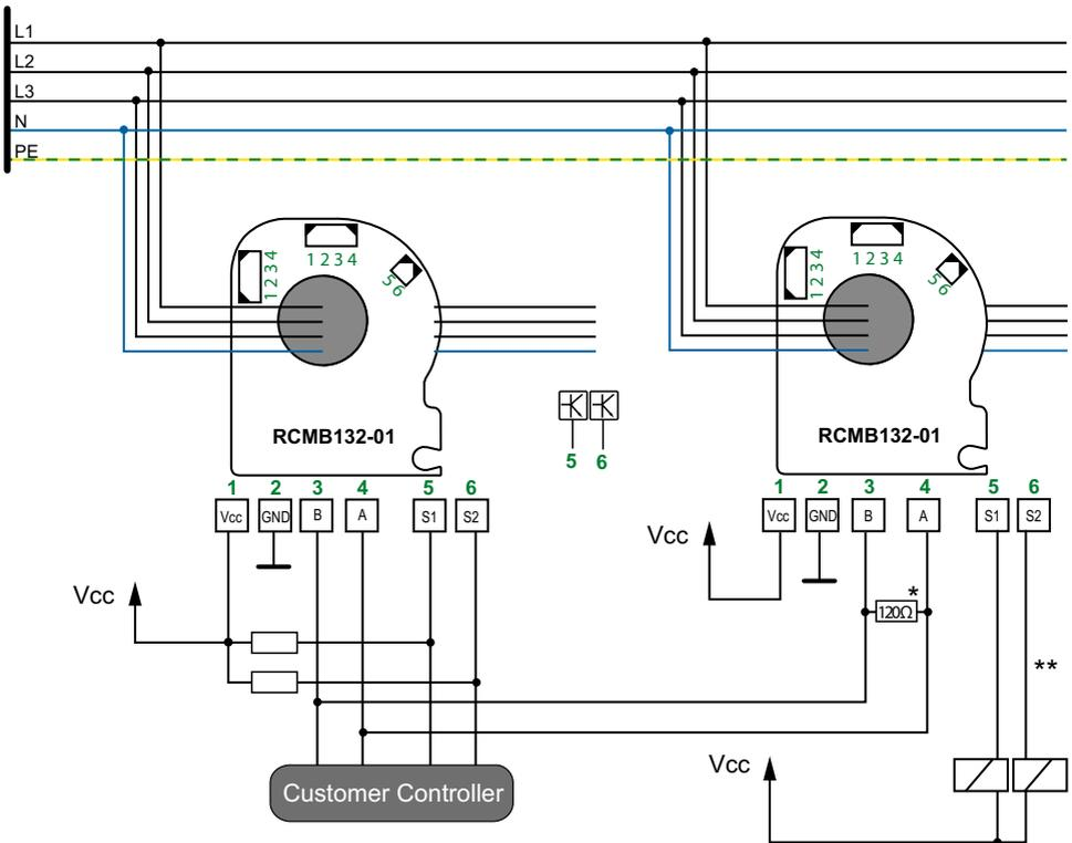
\* Terminating resistor 120 Ω must only be set on the last device in the RS-485 bus chain
