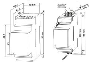
The front plate cover is easy to open at the lower part identified by an arrow.
